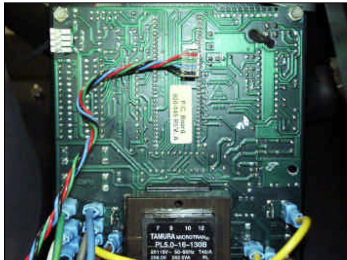
Figure 1: RS232 Adapter Cable connected to the control board.
